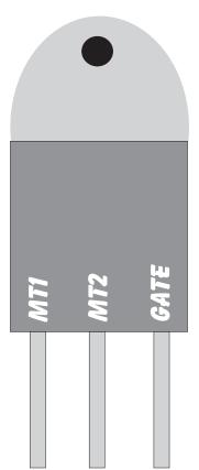
Using a ohmmeter gate to MT1 should read about 40 ohms both ways. If it doesn't read zero or infinity it is probably ok. The AC current flows from MT1 to MT2. Using the meter the MT1 to MT2 reading should be infinity either way. If the triac reads zero between these two pins then the triac is shorted. Gate to MT2 should also read as an open connection.
